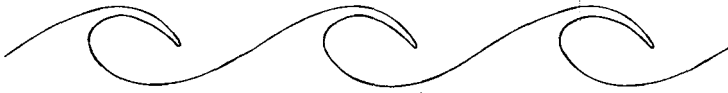
FIGURE 7. Sketch of a spatially periodic breaking wave. The curve is a constant-vorticity contour, \Omega_i = 0.1 for c_i A^{-1/2} = 0.4 .
